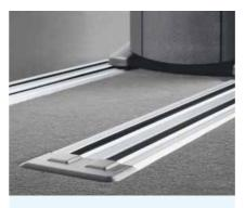
Rail system The rail system with roller mountings operates smoothly and extends along the length of the rear passenger compartment. It offers infinite positioning of the rear single seats, 3-seater bench seat and the multi-functional table.
